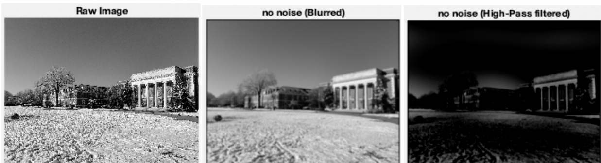
Figure 9: Raw Image (left), Blurred Image (middle), and Deblurred Image Using High-Pass Filter (right)
