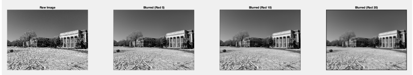
Figure 3: Raw Image (left) Compared with Blurred Image with Circular Averaging Filter of Size 5 (middle left), 10 (middle right), and 20 (right)
