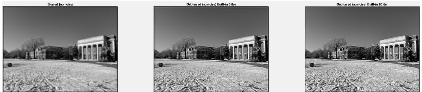
Figure 10: Blurred Image (left), and Deblurred Image Using Matlab Built-in Filter in 5 Iterations (middle), and 20 Iterations (right)
